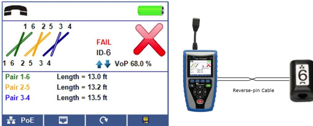
For any flat-satin or twisted-pair cable in a reverse-pin configuration, ignore the "FAIL" result and make sure that the wire-map is the same for each cable that you are testing.
